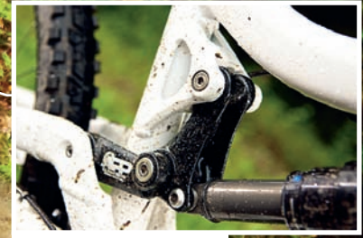
The new APP swing link produces a variable shock rate
