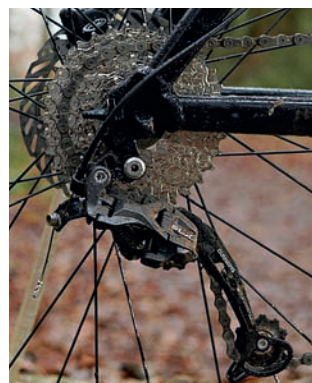
The 9-speed may look like last season's choice but 10-speed only offers some slightly closer-spaced ratios in reality
